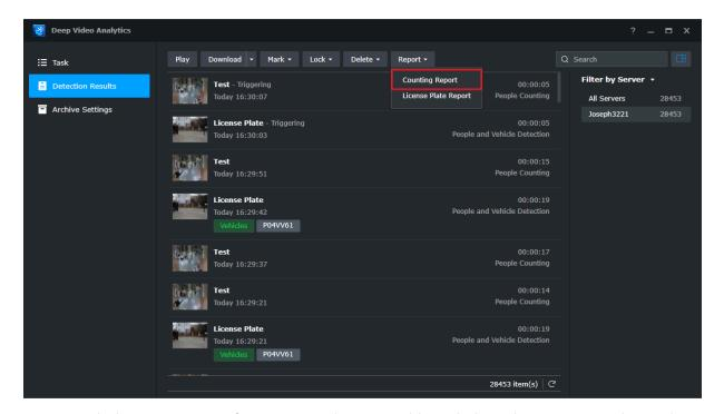
Reports will list the number of people entering and exiting within a given date and time. With the flexible display design, you can easily adjust the time range from daily to yearly. Data from different tasks can also be shown simultaneously to accommodate spaces with multiple entrances. If you wish to save a copy of the report, click **Export** to download it as an HTML or Excel file.
