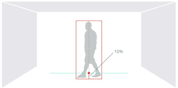
The detection line should be located on the ground, in the center of the camera screen, and span the entire width of the passage. If the line is drawn too short, people might pass through the entrance without crossing over it and be missed. The maximum length is 4 meters long.
