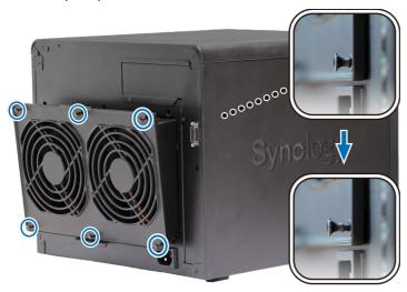
**3** To remove the malfunctioning fan module, you simply need to pull it out from your expansion unit.
