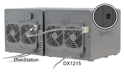
• If the DEFAULT/MANUAL switch is switched to MANUAL, press the POWER button located on the front panel to power on the expansion unit.
