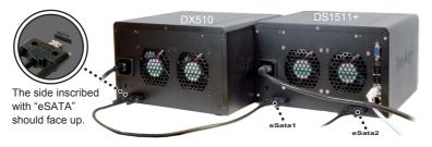
After the connection is complete, DX510 will be turned on or off automatically when the connected DiskStation powers on or off.
