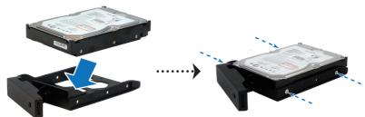
For 2.5" Hard Disk: Place the hard disk in the rectangular area (shown below) of the hard drive tray, turn the tray upside down, and then tighten the screws to secure the hard disk.
