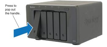
3 Pull the handle to remove the hard drive tray from DX510.
