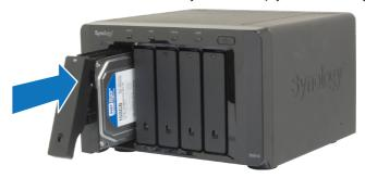
*Important:* Make sure the tray is pushed in all the way. Otherwise, the hard disk might not be able to function properly.
