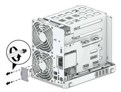
7. Remove the four screws securing the other PCle expansion shield in place, then the shield.
