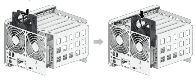
3. Install the backplate screws and connect the fan connectors in their corresponding slot as shown below.
