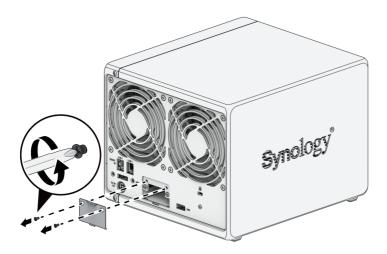
3. Insert the network upgrade module and tighten the two screws to secure the newly inserted module.
