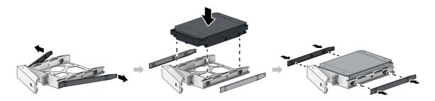
• For 2.5" drives: Remove the fastening panels from the sides of the drive tray and store them in a safe place. Place the drive in the area of the drive tray indicated in the image below. Turn the tray upside down and tighten the screws to secure the drive in place.
