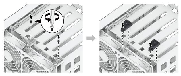
6. Remove the two screws as well as the PCle expansion shield beneath the fans at the back of your Synology NAS.
