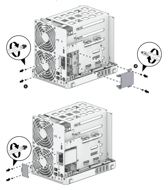
5. Re-install the plastic fan supports and their screws.
