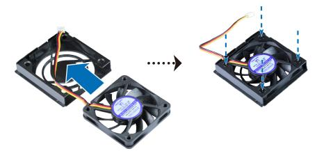
**6** Plug the fan power cord into the DiskStation, as illustrated below.
