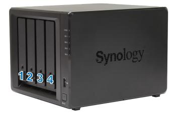
**Note:** If you want to create a RAID volume, we recommend that all installed drives are of the same size to make the best use of drive capacity.
