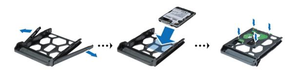
**4** Make sure the side marked with "**UP**" is facing up, and insert the hard drive tray into the empty hard drive bay. You should hear a click when the tray is locked in place.
