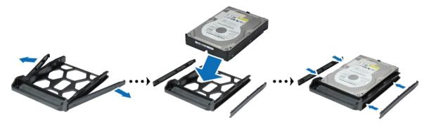
• For 2.5" Hard Disk:Remove the fastening panels from the sides of the hard drive tray and put them in a safe place. Place the hard disk in the blue area (shown below) of the hard drive tray, turn the tray upside down, and then tighten the screws to secure the hard disk.
